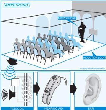
In 1987 [Ampetronic](#) was established and began to rapidly develop the technology in the UK. In 1991 Ampetronic developed the first '[phased array](#)' systems (multiple induction loops operating together out of phase to create constructive interference) capable of covering large areas in modern buildings with metal construction and/or to control spill.
