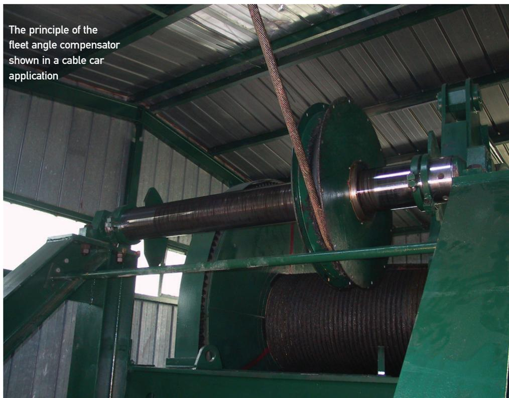
The principle of the fleet angle compensator shown in a cable car application
