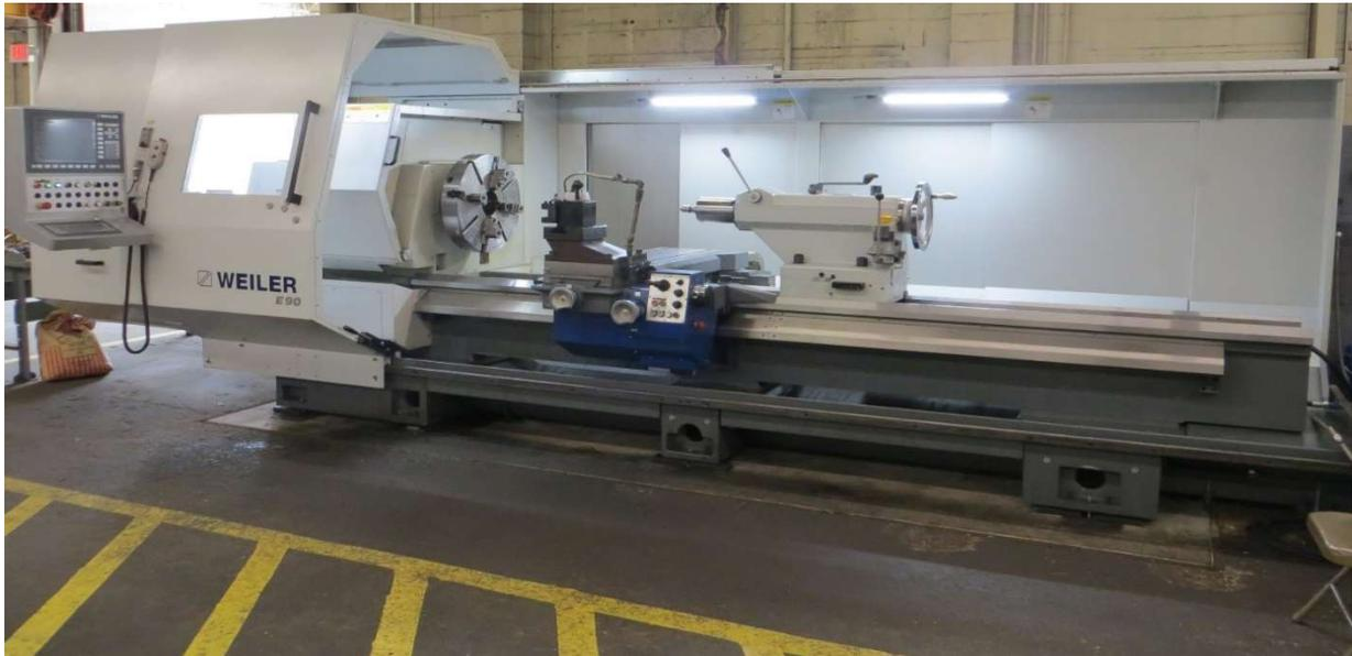
The Weiler E90 can turn cylinders up to 20" in diameter and up to 118" in length. This machine being smaller than the other Weilers has even easier accessibility and therefore easier operation. With the better accessibility and easier operation, it can turn out the jobs it is capable of faster than the larger machines.
